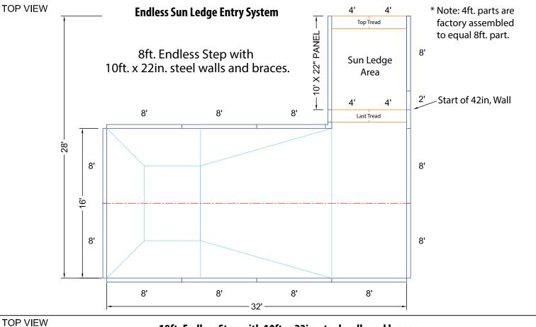
18ft. Endless Step with 10ft. x 22in. steel walls and braces.
